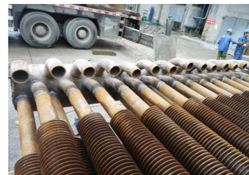
余热发电管束的翅片管间距离调整 Distance adjustment for the waste heat power generation pipe bundle's fin
