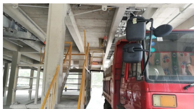
工厂整改后的水泥包装装车安全平台 The safety platform of the cement packing and loading after the rectification of the factory
